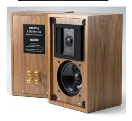
Built under license from the BBC the Stirling Broadcast LS3/5a V2 represents our first design collaboration with Derek Hughes. The LS3/5a V2 combines custom versions of modern high quality drive units with a high quality crossover, all housed in thin wall (9mm) damped construction birch plywood cabinets with screw-on removable front and rear panels which are fitted with double layers of bituminous pads.
